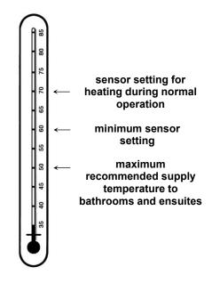
We recommend and it may also be required by regulations that an approved temperature limiting device be fitted into the hot water pipe work and serving a bathroom and ensuite when this water heater is installed. This will keep the water temperature below 50°C at the bathroom and ensuite. The risk of scald injury will be reduced and still allow hotter water to the kitchen and laundry.
