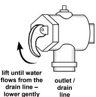
Operate the easing lever on the temperature pressure relief valve and expansion control valve once every six (6) months to clear any deposits and ensure the valve and its drain line are not blocked. It is very important the lever is raised and lowered gently. Refer to "Minor Maintenance Every Six Months" on page 16.
